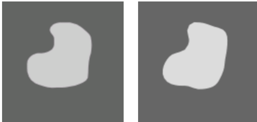
Figure 3. An optimisation achieved with the BIE with the diagram shown in Fig. 2. Three noisy projections of the original object (left) are available, making this a very difficult reconstruction problem. The image on the right represents the shape that minimises the minus-log-posterior on the right in Fig. 2, obtained by varying the 120 parameters that describe its geometric boundary.
